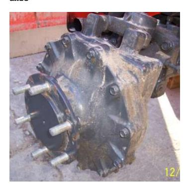
Now is a good time to test fit the spacer to the Axle & then to the wheel rim. The spacer should make full contact to the axle & the nuts/lug bolt has full tread contact , it's much easier to sort any problems without having anything bolted down.
